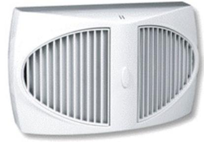
The design is such that the cross-current sections inside the fan ensure the two air streams are always kept separate preventing the incoming fresh air from being contaminated by the outgoing stale air.
